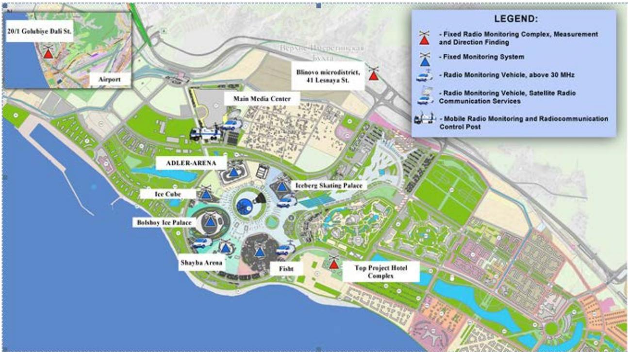
Figure 6: Arrangement diagram of the Sochi 2014 Automated Radio Monitoring System elements in the territory of the Coastal Cluster
