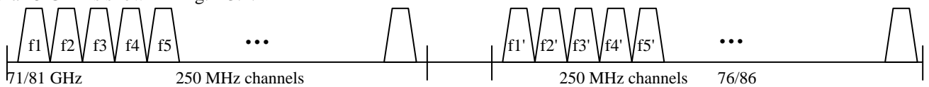
Fig. A3.2. Combining the channels from single 71-76 GHz or 81-86 GHz band into an FDD arrangement with duplex separation of less than 5 GHz
