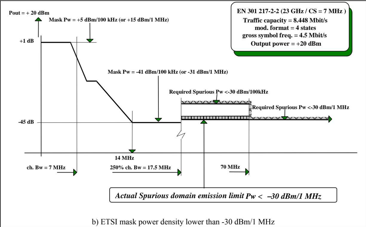
b) ETSI mask power density lower than -30 dBm/1 MHz
