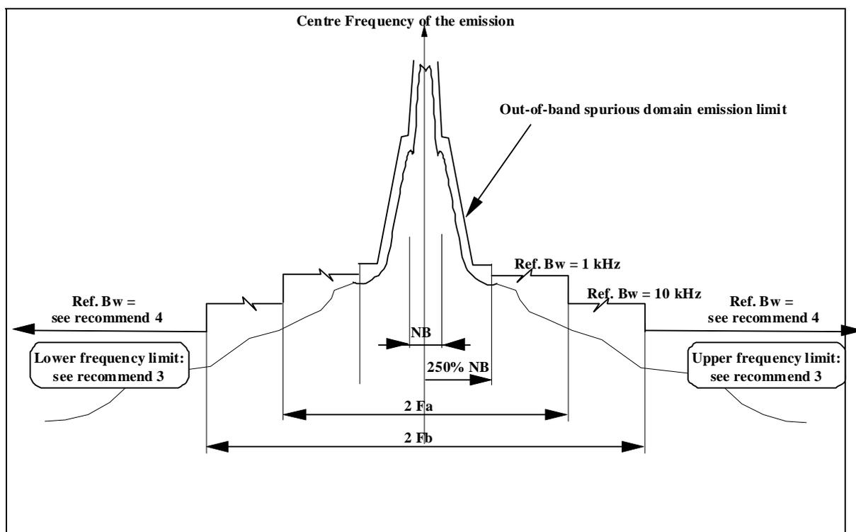
**Figure 2.1: Specific mask for spurious domain emissions for mobile services operating between 30 MHz - 1 GHz (see Table 2.2)**
