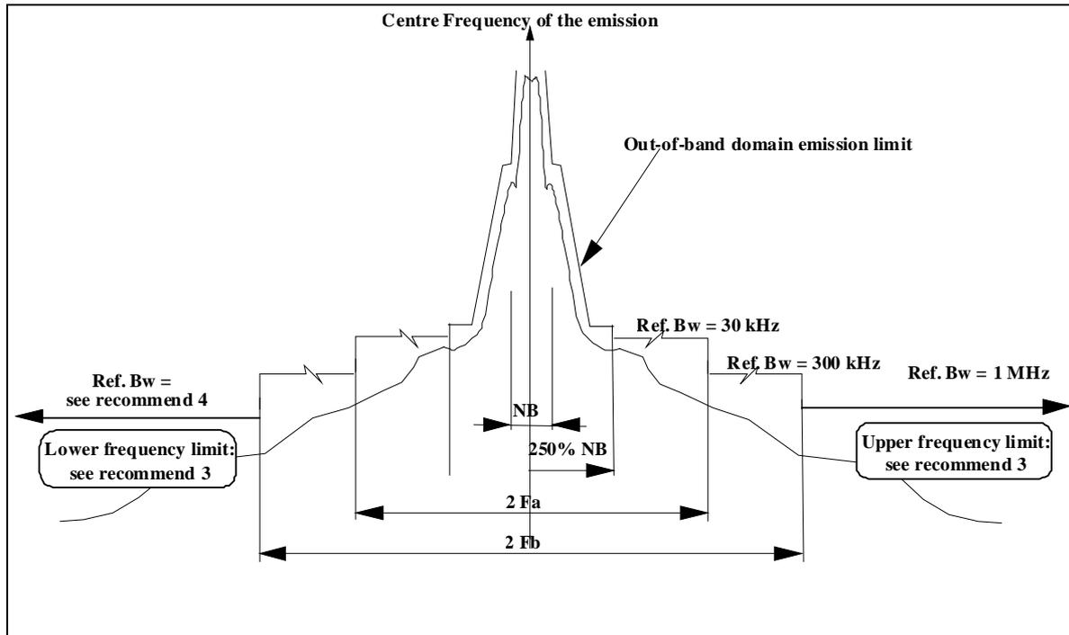
**Figure 1.2: Specific mask for spurious domain emissions for BWA systems operating between 1 GHz and 6 GHz**
